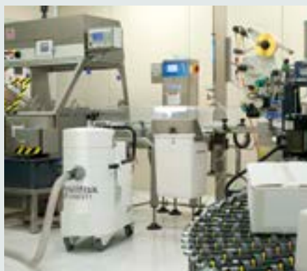
Recovery of waste from a packaging machine
